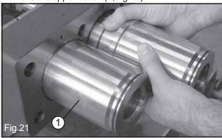
Once head and collector are removed the cylinders 1, Fig.21 are free to be taken out of the pump body. Beating the cylinders all around with a plastic hammer helps to loose them from possible scaling or deposit accumulated during operation.
