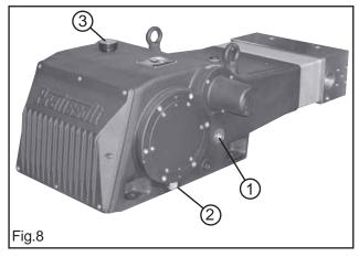
If necessary, top up from the oil plug 3, Fig.8.
