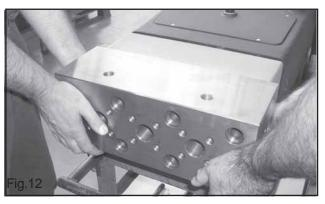
Remove the pump head (Fig.12).
