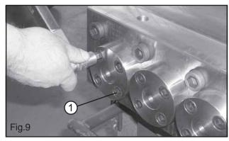
In order to have access to the delivery valves loose the 12 valve cover screws (1, Fig.9) and remove the valve covers
