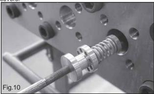
Once removed, take out the delivery valve guide with the spring and valve disk. An M10 threated bolt to be used as a simple extractor would help the operation (see Fig.10).
