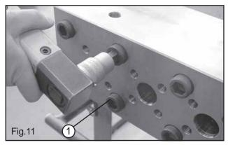
Loose and remove the 8 head screws (1 Fig.11).
