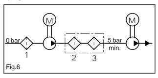
The filters should be installed as close as possible to the pump, allow easy inspection and have the following specifications:
