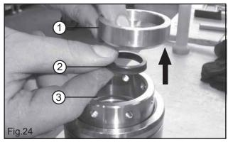
Remove the rear seal support 1, the rear seal 2 and the O'ring 3, Fig.24.
