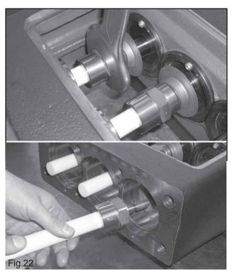
Once the cylinders are removed, loose the plungers and check them for wear (Fig.22). Replace if necessary.
