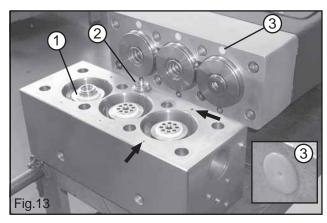
When removing the head from the pump pay attention to the valve seats (1, Fig.13) and the suction valve disks (2 Fig.13) which may fall off the head.
