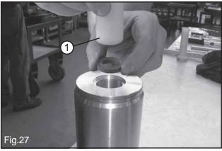
Each pressure packing set component should fit tight in the cylinders because of a little interference designed in the ext. diameter. A pin of adeguate dimensions (1, Fig.27) helps in guiding each component straight and alligned all the way down in the cylinder.
