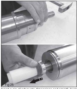
Insert a pin of adeguate dimensions and smartly beat till the complete pressure packing set is out (Fig.25). Replace pressure packing set at every inspection.
