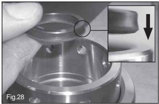
The new rear seal should be mounted with the larger diameter side first in, as shown in Fig.28.
