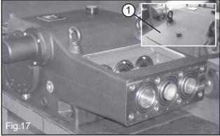
Remove the upper cover by loosening the four screws (1, Fig.17).
