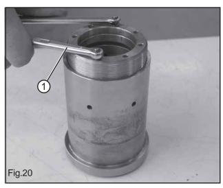
Disassemble the packing support from the cylinder by means of a pin key (1,Fig.20).
