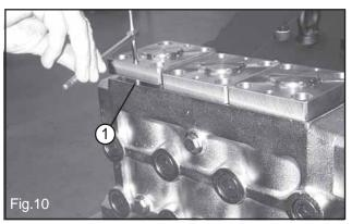
Tighten the two grub screws 1, Fig.10 of each valve cover till the complete valve unit moves upwards enough to allow easy extraction.
