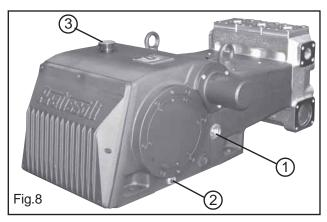
If necessary, top up from the oil plug 3, Fig.8.
