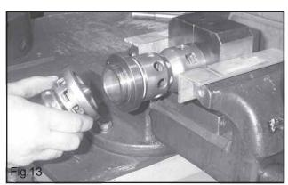
Check the valve components for wear and replace where necessary.
