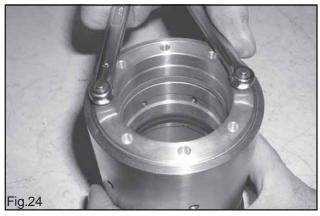
Set up the complete package without tightening the packing support (1, Fig.24) but making sure that the pressure packings snap in place.
