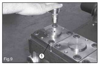
Loose and remove the valve cover screws 1, Fig. 9.
