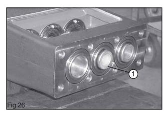
Fit the pumping units back in the pump cranckcase (1, Fig.26).
