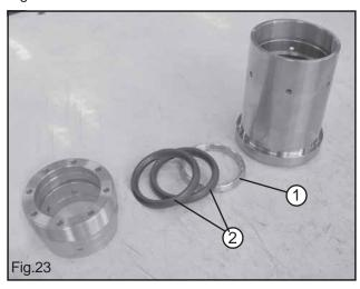
Before re-assembling the pumping unit carefully clean the pressure packing seat in the cylinders, fit in place the packing ring (1, Fig.23) and then the pressure packings (2, Fig.19). A little bit of grease helps sliding the packings into the packing support.
