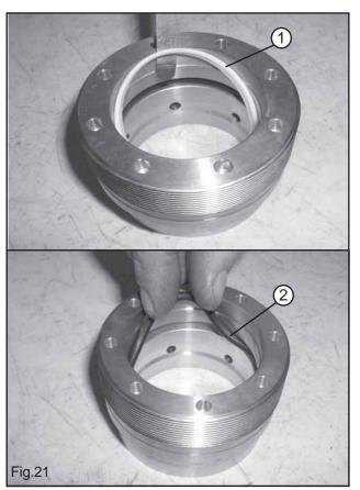
Remove scraper (1, Fig.21) and O'ring (2, Fig.22) from the packing support.
