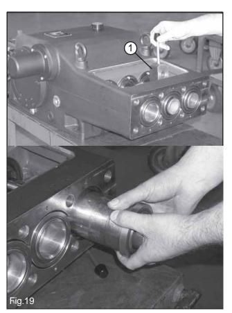
Push the plungers forward by rotating the crankshaft, then introduce our tool p/n 2000.3006.0 (or equivalent) (1, Fig.19) in between the piston guide and the cylinder. With the tool in place, rotate the crankshaft until the cylinder is pushed out together with the plungers. (Fig.19).
