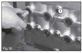
For inspecting the pumping unit remove the head by loosening the eight head screws (1, Fig. 16).
