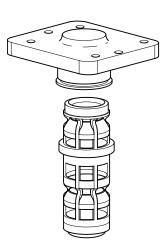
Valve components of each valve unit are screwed together in one single block and therefore they can be easily serviced, replaced and installed back in place. Separating the various components of the valve unit is carried out by means of simple tools as shown in Fig. 11, 12, 13 of the next page.
