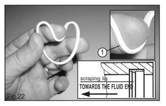
In order to fit the new scraper in place shape it manually as shown in Fig.22.
