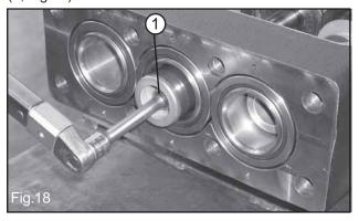
Loose and remove the plungers screws (1, Fig.18).
