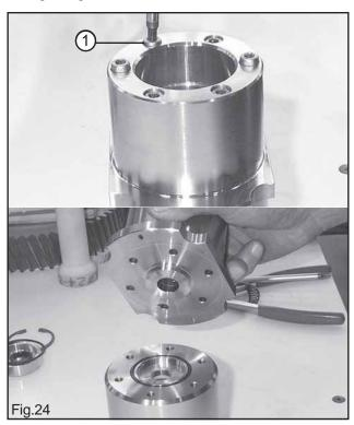
Remove the 6 packing support screws (1 Fig.24).
