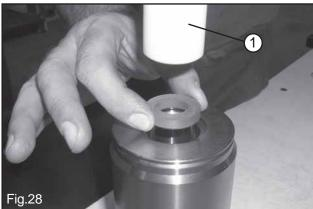
Each pressure packing set component should fit tight in the cylinders because of a little interference designed in the ext. diameter. A pin of adeguate dimensions (1, Fig.28) helps in guiding each component straight and alligned all the way down in the cylinder.
