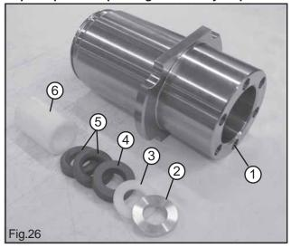
Reassemble packing support and cylinder. Screws 1, Fig.26 should be tighten with a torque wrench set for 1,7 Kgm.Fit each new component of the pressure packing set in the cylinder making sure of the correct order as shown in Fig.26 and Fig.27:
