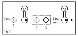
The filters should be installed as close as possible to the pump, allow easy inspection and have the following specifications:
