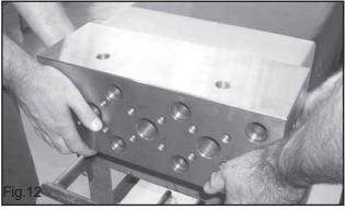
Remove the pump head (Fig.12).
