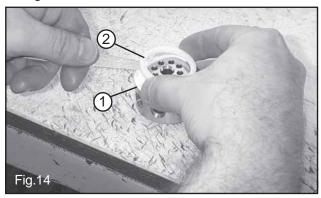
Remove the valve seats (1, Fig.14) from the head, check them for wear and replace if necessary.
