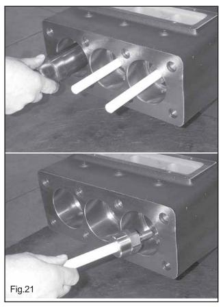
Once the cylinders are removed, loose the plungers and check them for wear (Fig.21). Replace if necessary.
