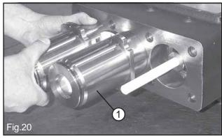
Once head and collector are removed the cylinders are free to be taken out of the pump body.
