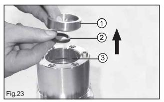
Remove the rear seal support 1, the rear seal 2 and the O'ring 3, Fig.23.
