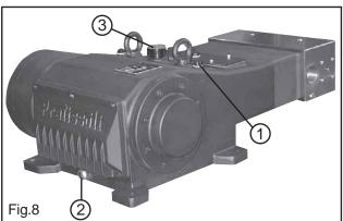
If necessary, top up from the oil plug 3, Fig.8. Check the oil when cold and change the oil when still hot (pump still at working temperature).
